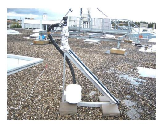
To these belongs for example a special solar liquid test bed. With this solar liquid test bed different heat transfer liquids can be checked for its temperature stability up to 300°C. All such high temperatures appear for example in directly perfused evacuated tube collectors.
